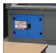
Flammable/corrosive chemical safety cabinet
